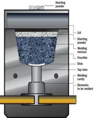
View of a vertical section of the mould
