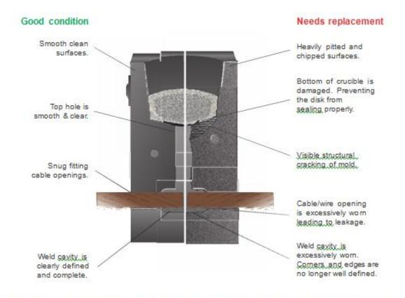
NOTE: Inspect the mold regularly to determine if a mold should be replaced.
